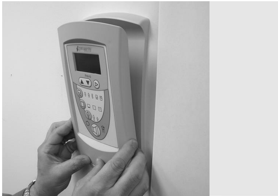
Figure 41 Snapping the Operator Panel to the Mounting Cradle
